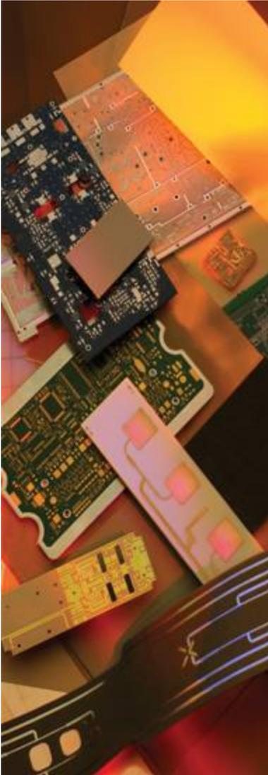
Arlon 92ML ceramic filled thermally conductive multifunctional epoxy laminate and prepreg products are provide best-in-class thermal performance with increased thermal conductivity of 2 W/mK for multilayer PWB's for applications requiring thermal management throughout the entire board volume.
